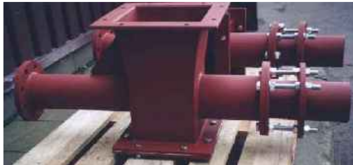
Abb.14: Ejector DN80 for Conveying of flue ash
