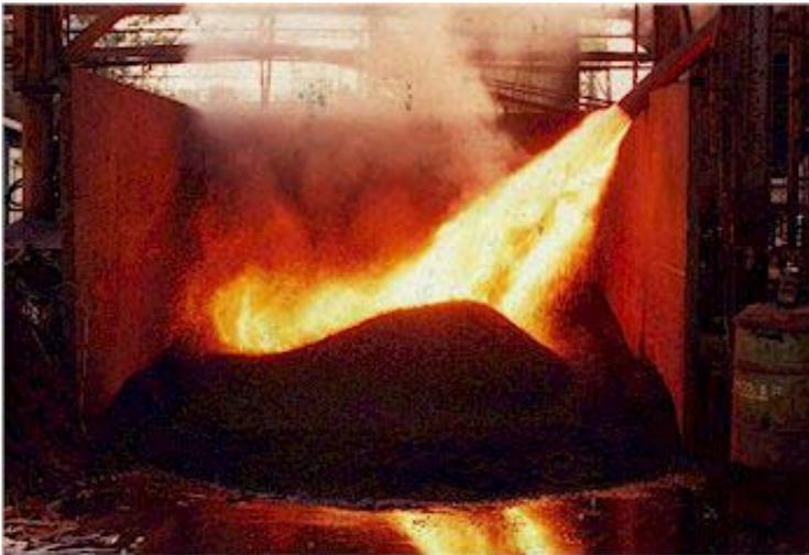
Heat losses have to be kept to a minimum as the expected temperature of sponge iron at the melt shop should be kept above 400 eC and the percentage of fines generated should be kept below 10 % for the system to be profitable.
